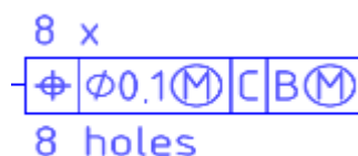
Figure 5. Geometric tolerance annotation with qualification note ('8 holes')
